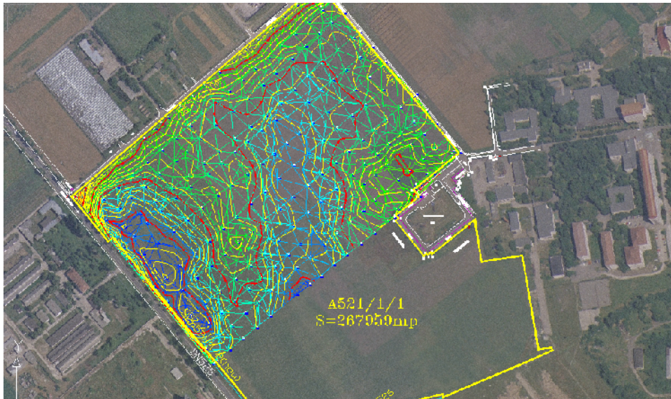
Figure 6 - TIN model and level curve overlapping the ortophotoplan
