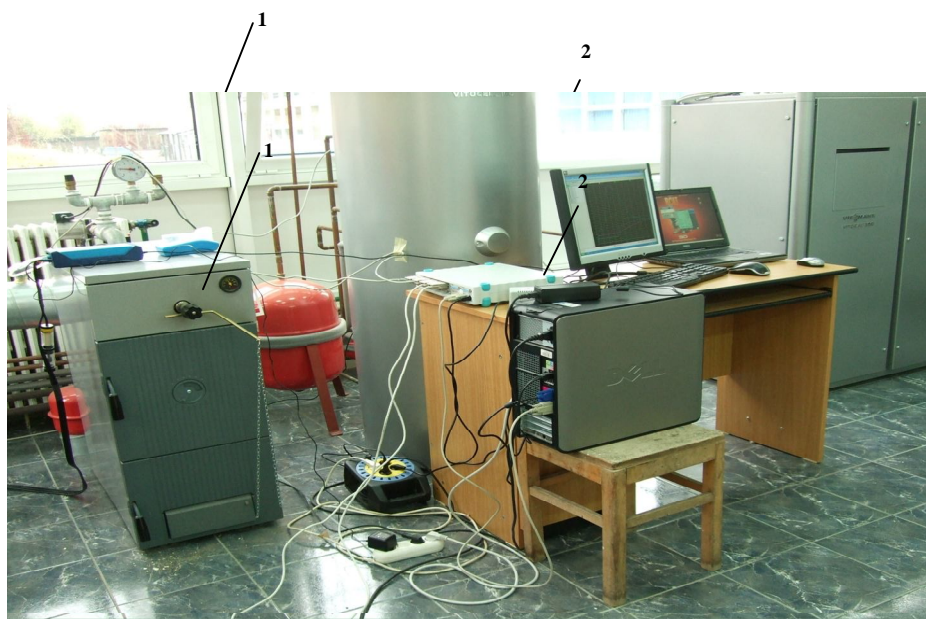
Figure 1. Test bench: 1 – boiler and heating system; 2 – data acquisition system
