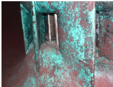
Figure 7. Photo of the spiral case, the stator columns and of the guide apparatus
