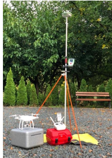
Figure 2. System GNSS Leica GS 08, Drone-Dji Phantom 4, GCP (Ground Point Control)
