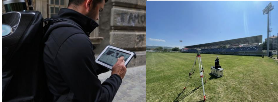
Figure 3. Leica Pegasus: Backpack and Leica Viva GS14 (Master Base) – Lipova Stadium
