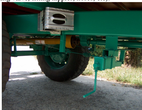
Figure 6. Parking braking, wheel chock, intermediary transmission
