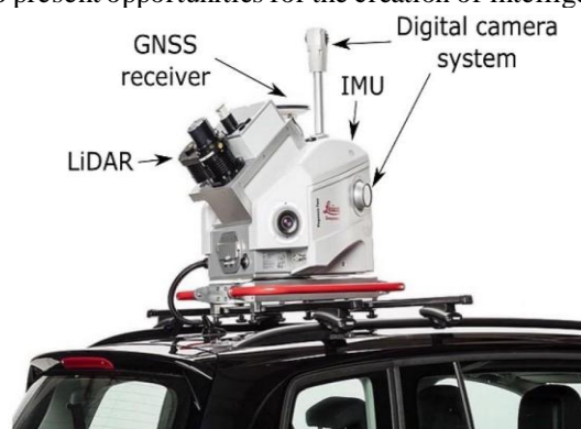
Figure 9. Mobile Mapping System with LiDAR and GNSS Components
