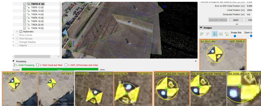
Figure 15. Example of marking the correct position of several GCPs
