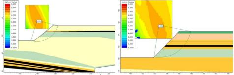
Figure 6. 2<sup>nd</sup> step of the quarry (left); 4<sup>th</sup> step of the quarry (right) - the critical sliding surface
