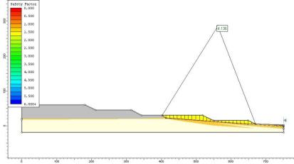
Figure 8. System of steps I-II of the inner dump - the polygonal sliding surface defined at the contact between the base terrain and the inner dump (at average -  $\sigma$  values of the geotechnical characteristics of the sterile rocks)
