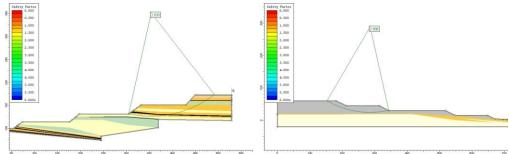
Figure 7. System of steps of the quarry III-IV (left); System of steps of the inner dump III-IV (right) - the sliding surface through the foot of the slope
