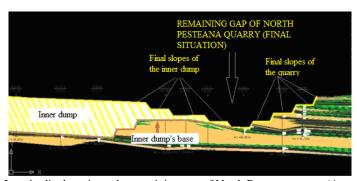
Figure 2. Longitudinal section - the remaining gap of North Pesteana quarry (APOSTU, 2018)
