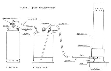
Fig. 2. Main units of the soil generator used by NEFELA: air tank (1), solution tank (2) and incinerator (3)
