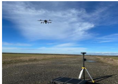
Figure 3. DJI 300 RTK matrix with D-RTK 2 GNSS mobile station
