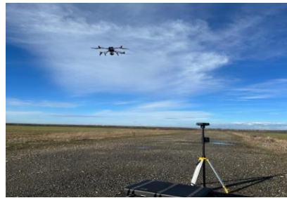
Figure 6. DJI 300 RTK matrix with D-RTK 2 GNSS mobile station
