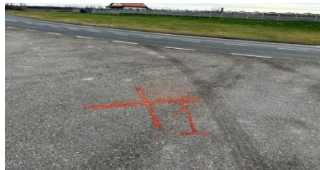
Figure 5. Image with ground marking for GPS control determinations
